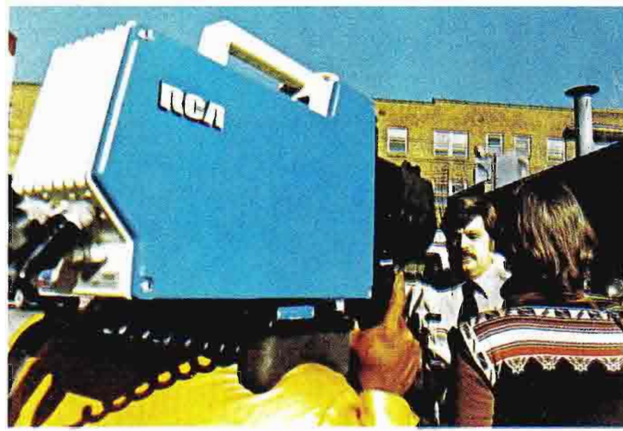
The TK-76 travels in style, in its own protected case. The camera's sensitivity and ability to operate at low light levels enhances its usefulness for ENG.
