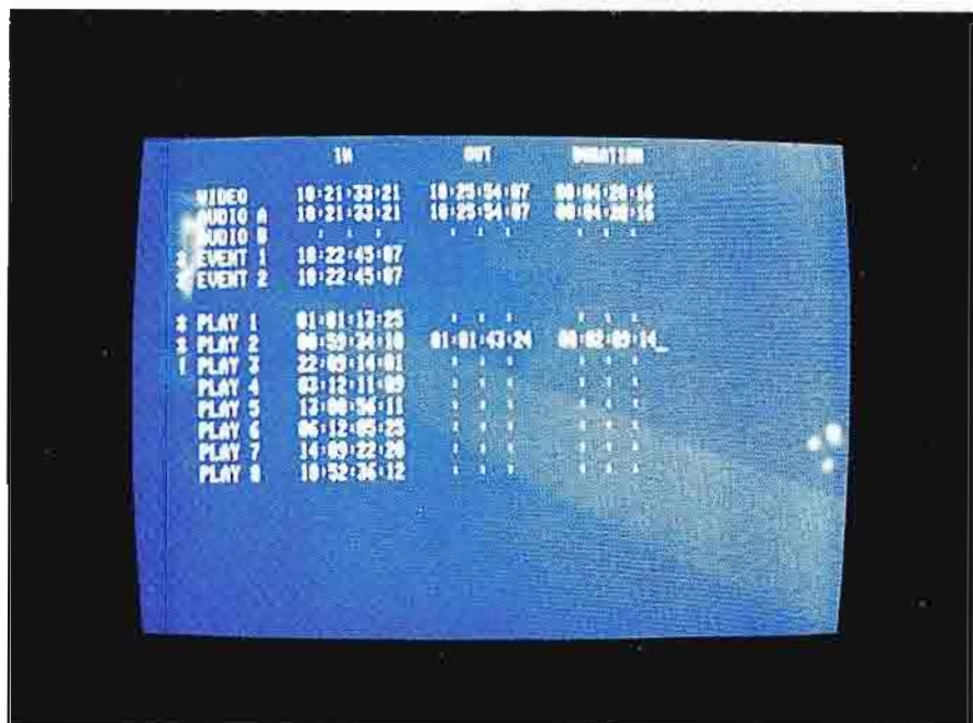
External monitor display provides a visual display of individual "In", "Out" and "Duration" times for all machines in the system.
