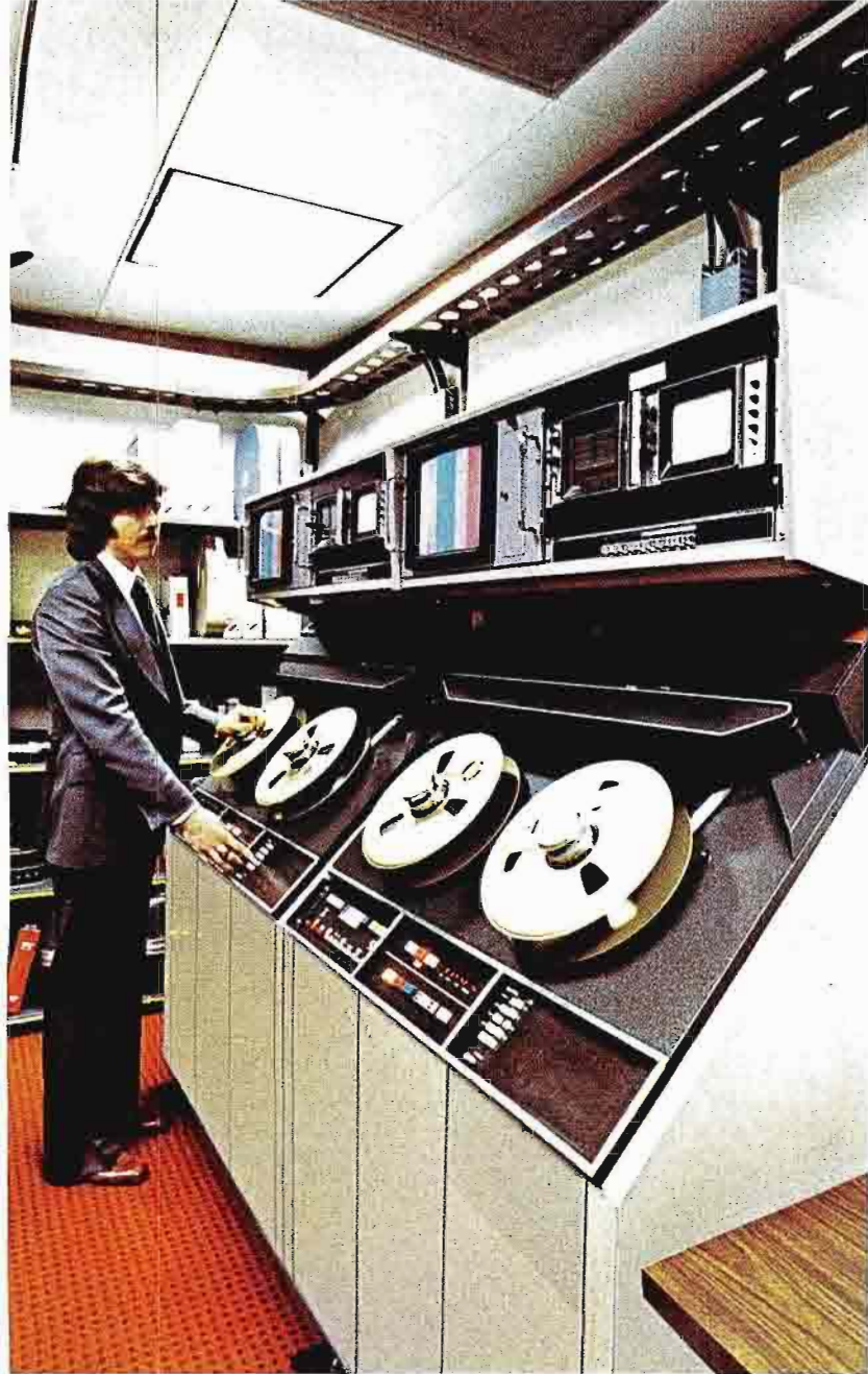
Chief Engineer Pat Howley operates TR-600's in Merrill Lynch video production facility. Quad machines are used for mastering, with edited tapes dubbed to videocassette format for distribution.
