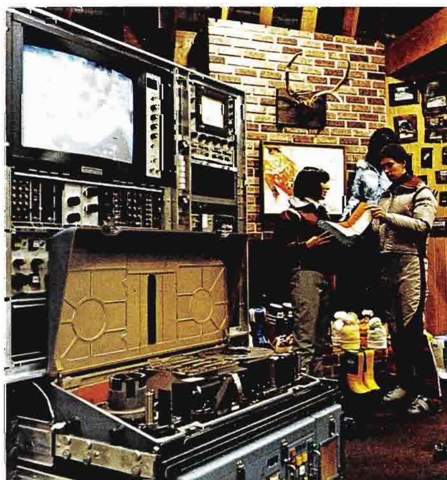
TPR-10 portable quad VTR used with "Minimote" permits immediate playback in color to determine if a new "take" is needed.
