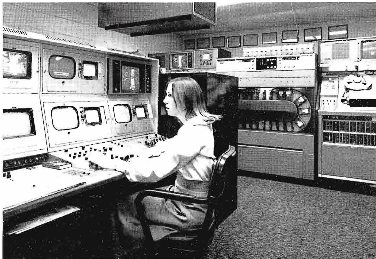
Master Control operator at TV-20 handles on-air switching, loads TCR-100 "cart" machine and TR-70 VTR and shades film cameras when necessary.
