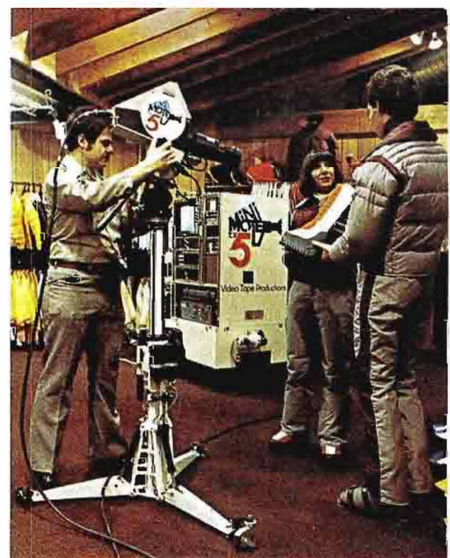
TKP-45 portable color camera used with "Minimote". Its automatic features and light sensitivity make it ideal for indoor and outdoor shoots.
