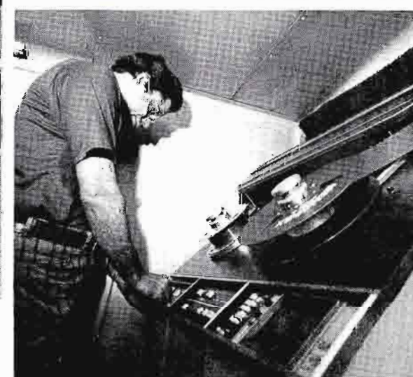
TR-600 mounted inside TV-20 van provides top quality recordings. One engineer handles the taping operation and shades camera on remotes.
